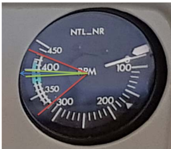
Figure 8 – N_R range limitations in flight (green) and autorotation (red)
