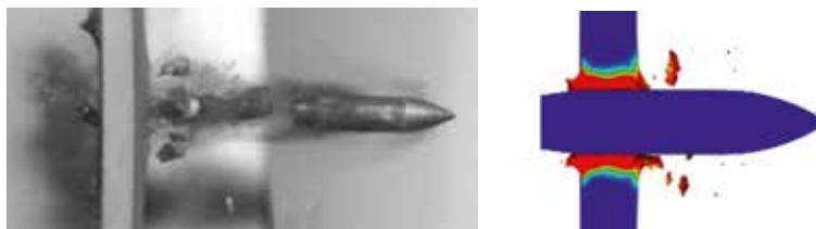
Figure 1: Comparison of experimental test and numerical simulation of a 7.62 mm AP bullet perforating a 5 mm thick AM AlSi10Mg plate [1].
