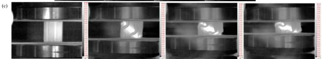
Figure 4 : Compressive behaviour of tri-hexagonal structure at 500 mm/min fabricated by SLM (a) : Force-displacement compressive curve; (b) : Images of the deformation process; (c) : Images of thermal change during compressive loading.
