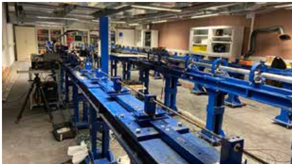
Fig. 1 – Experimental set-up: a) SHTB; b) heating system
