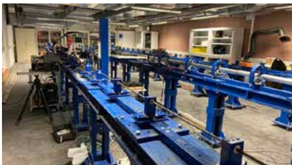
Fig. 1 – Experimental set-up: a) SHTB; b) heating system
