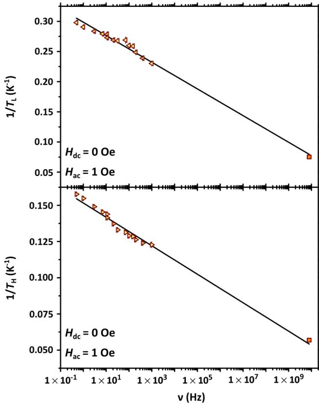
FIG. 6. Dependence of the inverse of  $T_L$  and  $T_H$  on frequency (upper panel and lower panel, respectively). The triangles and the squares refer to ac susceptometry and CPWR-based measurements, respectively. The continuous lines are best-fitting functions based on the activated trend reported in Eq. (5).
