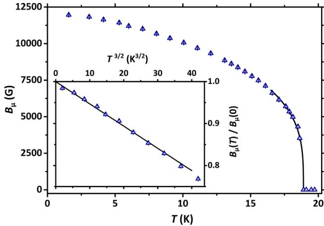
FIG. 2. Main panel: Dependence of the average local magnetic field at the muon site on temperature extracted from  $\mu$ SR data in zero-field conditions. The continuous line is a best-fitting curve based on Eq. (4). Inset: Blow-up of the average local magnetic field at the muon site at low temperatures normalized over its extrapolated value at zero temperature. The continuous line is a guide to the eye highlighting a dependence on  $T^{3/2}$ .
