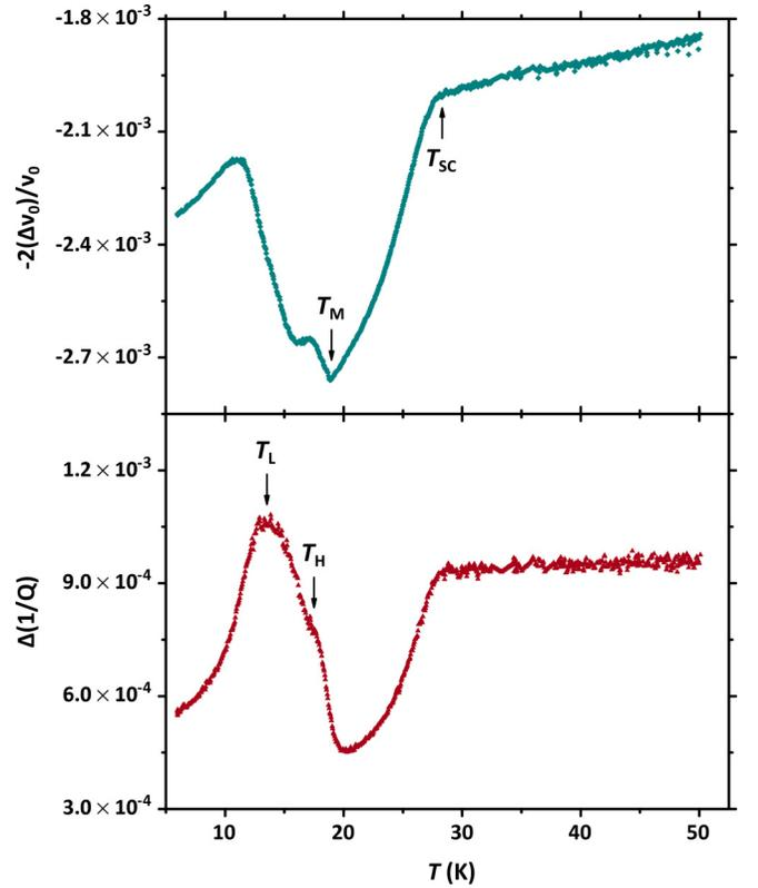
FIG. 5. Fractional shifts of the resonance frequency  $\nu_0$  (upper panel) and of the inverse quality factor  $1/Q$  (lower panel) of the CPWR due to the presence of the sample under test at  $\nu \simeq 7.9$  GHz. According to Eq. (1), these quantities are proportional to the high-frequency magnetic susceptibility real and imaginary parts:  $\Delta\nu_0/\nu_0 \propto \chi'$  and  $\Delta(1/Q) \propto \chi''$ .
