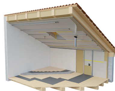
Barriera al vapore da https://www.riwega.com/ds-46-pe/
