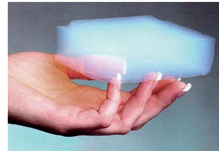
Aspetto aerogel, solido secco semitrasparente da https://nanografi.com/blog/promising-invention-in-the-insulation-industry-by-nanotechnology-aerogel/
