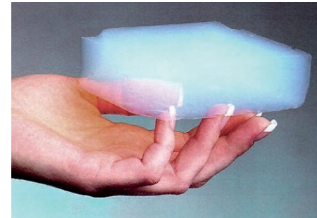
Aspetto aerogel, solido secco semitrasparente da https://nanografi.com/blog/promising-invention-in-the-insulation-industry-by-nanotechnology-aerogel/
