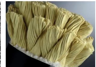
Fibre aramidiche da <https://www.universalinsulating.it/it/fibra-aramidica-16.asp>
