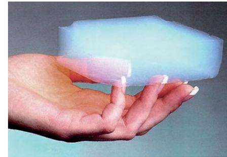
Aspetto aerogel, solido secco semitrasparente da <https://nanografi.com/blog/promising-invention-in-the-insulation-industry-by-nanotechnology-aerogel/>
