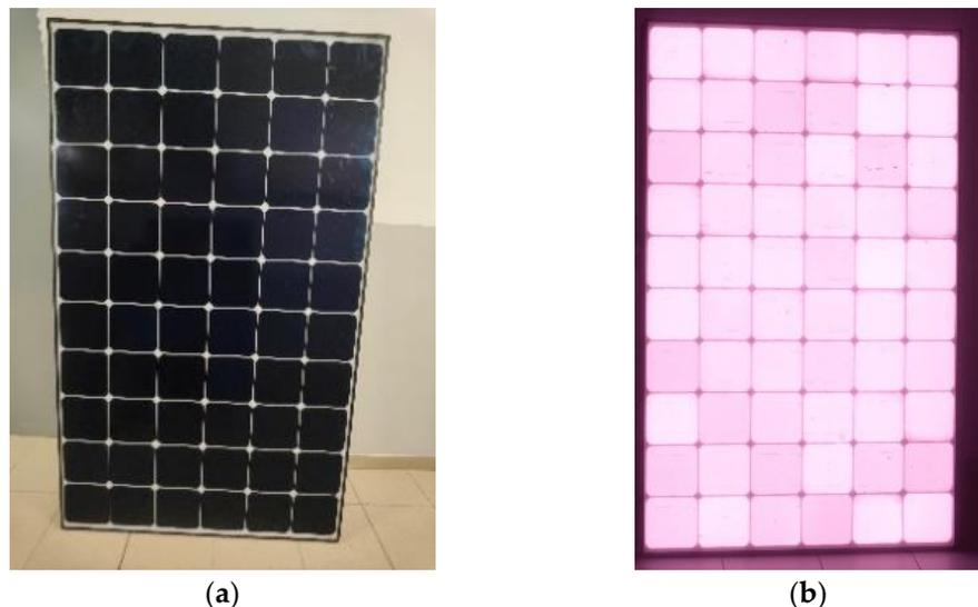
**Figure 4.** PV module under test in visible light (a) and during the EL test (b).
