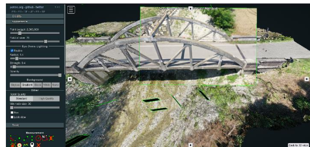
Figure 2. Example of a web-based interactive platform for exploring 3D products with oriented images developed with Potree solution.
