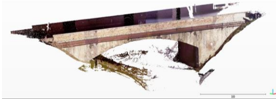
Figure 6. TLS point cloud of the Cortemaggiore bridge (Piacenza, Italy).
