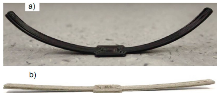
Figure 29: a) Distortion of FFF printed neat polypropylene part and (b) reduction of shrinkage and distortion by adding 30 wt.% hemp fiber to PP [164]
