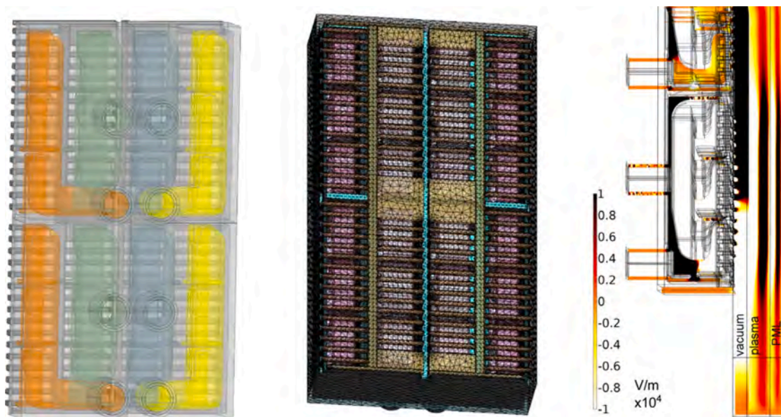
Fig. 18. Models for simulations of the reference TAH antenna: a) back view of the HFSS model with rerouting of the feeders visible; b) front view of the TOPICA model; c) side view of the RAPLICASOL model with radial RF electrical field representing fast wave.
