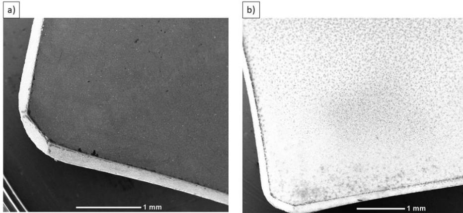
Fig. 2(color): EDS analysis on the near-edge region of SiC before (a) and after the corona treatment (b).
