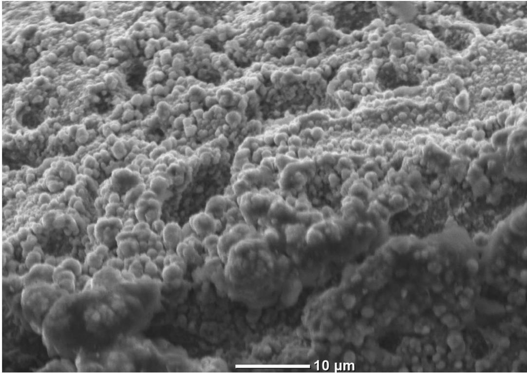
Fig. 5: Top view of the corona-induced silica layer visible after SiC exposure to the corona discharge system.
