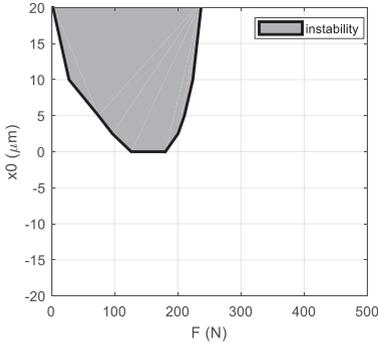
**Fig. 10.** Stability map as  $x_0$  varies:  $P_S = 0.5$  MPa,  $d_v = 0.5$  mm,  $d = 1$  mm,  $k_m = 1.8 \cdot 10^5$  N/m,  $V_1 = 1.4 \cdot 10^{-6}$  m<sup>3</sup>
