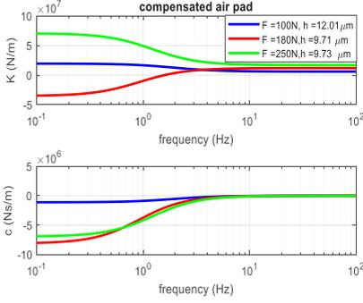
**Fig. 7a.** Compensated pad: dynamic stiffness and damping vs. frequency (from 0.1 Hz to 100 Hz).  $P_S = 0.5$  MPa,  $x_0 = -20$   $\mu\text{m}$ ,  $d_v = 0.5$  mm,  $k_m = 1.8 \cdot 10^5$  N/m,  $V_1 = 1.4 \cdot 10^{-6}$  m<sup>3</sup>
