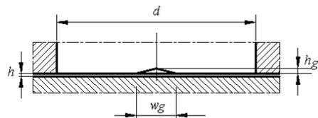
**Fig. 1b.** Supply hole cross geometry.
