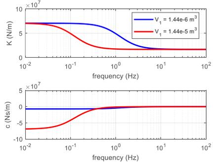
**Fig. 9.** Compensated pad. Dynamic stiffness and damping vs. frequency, effect of the volume  $V_1$ .  $P_S = 0.5$  MPa,  $x_0 = -20$   $\mu\text{m}$ ,  $d_v = 0.5$  mm,  $d = 1$  mm,  $k_m = 1.8 \cdot 10^5$  N/m,  $F = 250$  N,  $h = 9.73$   $\mu\text{m}$
