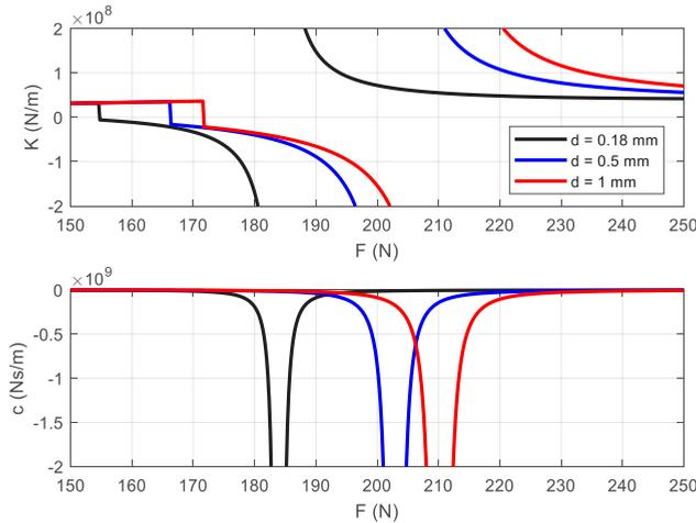
**Fig. 6.** Stiffness and damping of the compensated pad in static conditions, for some diameters  $d$ :  $P_S = 0.5$  MPa,  $x_0 = -20$   $\mu\text{m}$ ,  $d_v = 0.5\text{mm}$ ,  $k_m = 1.8 \cdot 10^5$  N/m.
