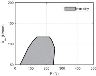
**Fig. 12.** Stability map as  $k_m$  varies:  $P_S = 0.5$  MPa,  $x_0 = -20$  μm,  $d_v = 0.5$  mm,  $d = 1$  mm,  $V_1 = 1.4 \cdot 10^{-6}$  m<sup>3</sup>
