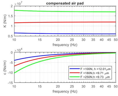
**Fig. 7b.** Compensated pad: dynamic stiffness and damping vs. frequency (from 10 Hz to 50 Hz),  $P_S = 0.5$  MPa,  $x_0 = -20$   $\mu\text{m}$ ,  $d_v = 0.5$  mm,  $k_m = 1.8 \cdot 10^5$  N/m,  $V_1 = 1.4 \cdot 10^{-6}$  m<sup>3</sup>
