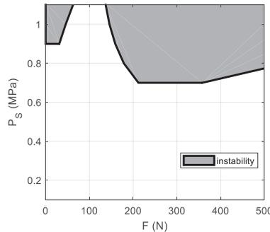
**Fig. 14.** Stability map as  $P_S$  varies:  $x_0 = -20$  μm,  $d_v = 0.5$  mm,  $d = 1$  mm,  $k_m = 1.8 \cdot 10^5$  N/m,  $V_1 = 1.4 \cdot 10^{-6}$  m<sup>3</sup>
