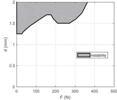
**Fig. 11:** Stability map as  $d$  varies:  $P_S = 0.5$  MPa,  $x_0 = -20$  μm,  $d_v = 0.5$  mm,  $k_m = 1.8 \cdot 10^5$  N/m,  $V_1 = 1.4 \cdot 10^{-6}$  m<sup>3</sup>
