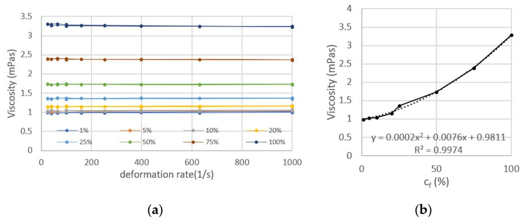
**Figure 7.** Characterization of the viscosity of the liquid generator. (a) For all the concentrations tested the viscosity has no dependence on the deformation rate (i.e., Newtonian liquid); (b) the viscosity bears a quadratic relationship to the surfactant concentration.
