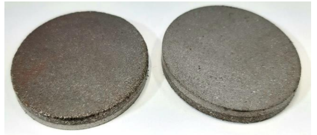
Fig. 5. Double-layer samples formed by bonded and hybrid magnets (on the left hybrid 70 % and on the right hybrid 40 %).
