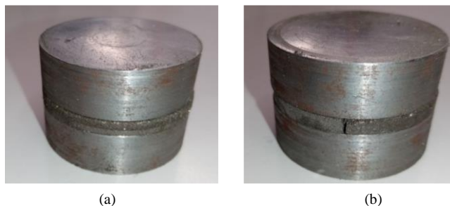
Fig. 9. Additional soft iron for produced samples, (a): series arrangement, (b): parallel arrangement.
