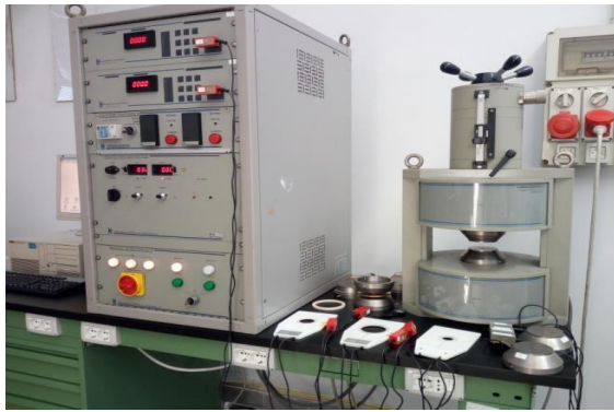
Fig. 7. The hysteresisgraph: view of the measurement system.
