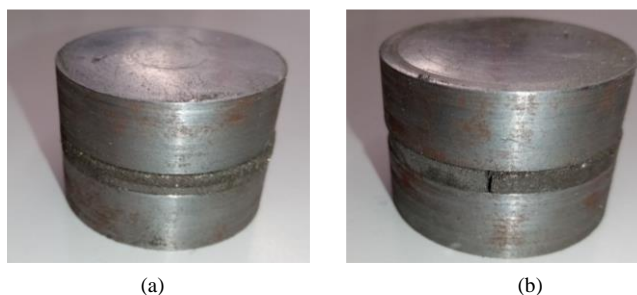
Fig. 9. Additional soft iron for produced samples, (a): series arrangement, (b): parallel arrangement.
