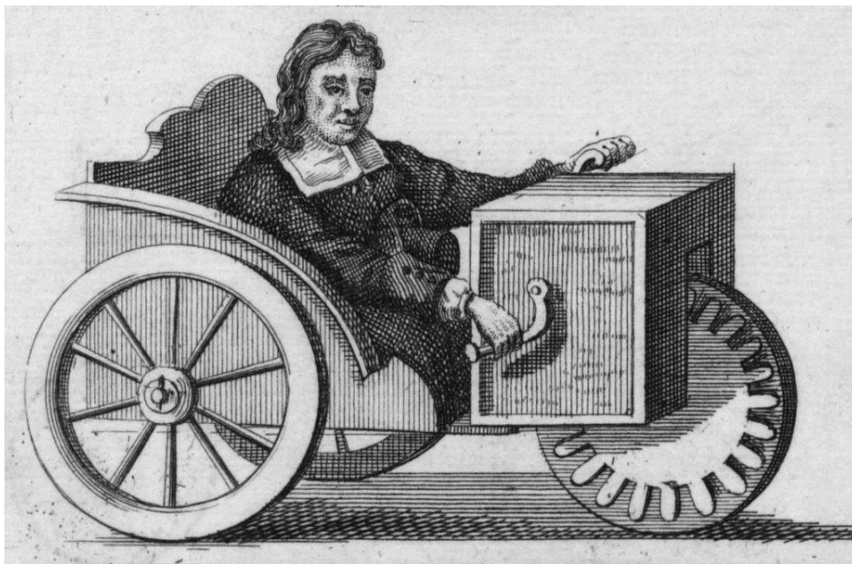
Figure 1.2: Representation of the first self-propelling vehicle for disabled The figure shows a three-wheeled vehicle in which the front wheel is propelled by cranks.
