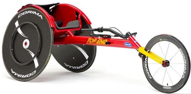
Racing wheelchair for sport with the handrim system [59]–[64]
