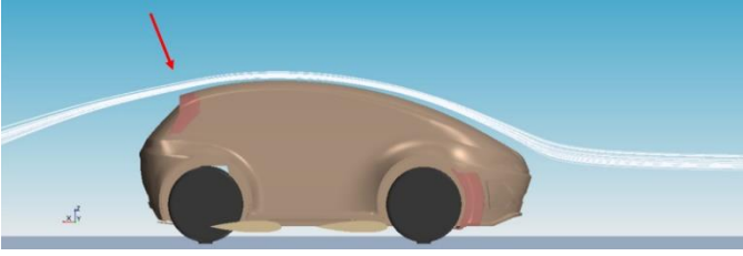
Figure 30 Complete configuration, JUNO streamlines scene CFD
