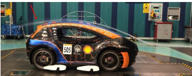
Figure 29 Complete configuration, JUNO's smoke wind tunnel test
