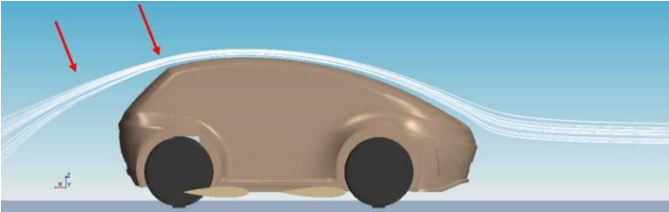
Figure 32 Standard configuration, JUNO's CFD streamlines scene
