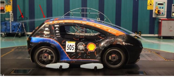
Figure 31 Standard configuration, JUNO's smoke wind tunnel test
