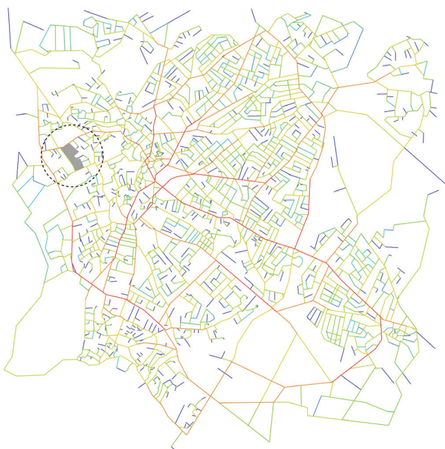
Figure 3. Segment Analysis showing the distribution of Normalised Angular Choice; segments in cooler colours have lower NACH values, while segments with warmer colours have higher NACH values.
