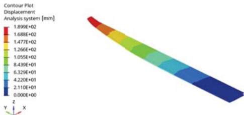
Fig. 14. Wing displacement in cruise conditions.
