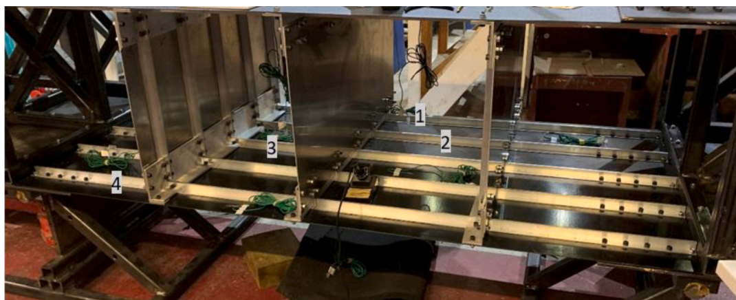
Fig. 13. Location of debonded stiffeners.
