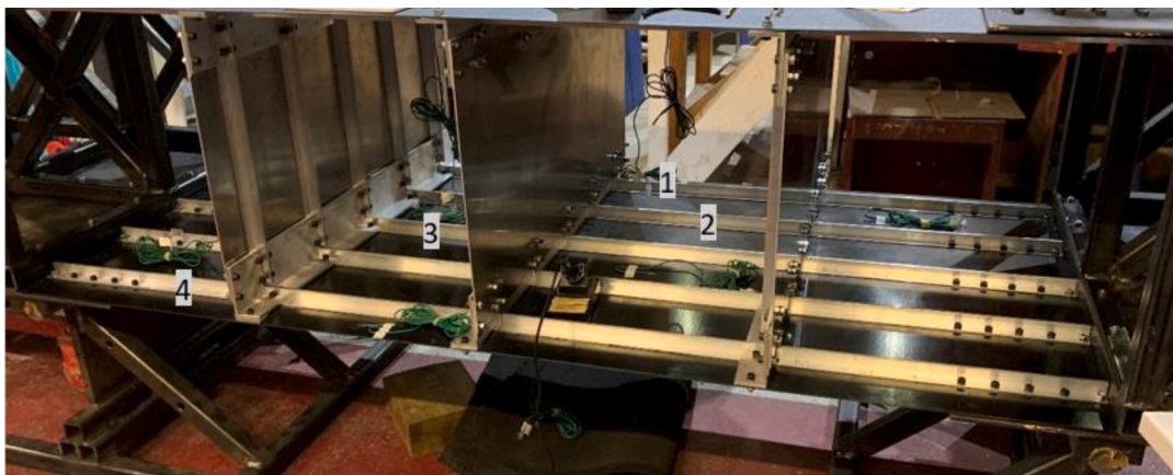
Fig. 13. Location of debonded stiffeners.
