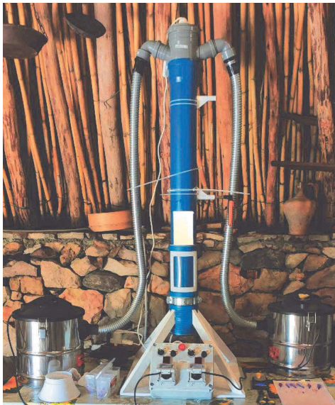
Fig. 2. Wind tunnel configuration, at the centre the main tube, with the windows opened, at the sides the two aspirators, at the bottom the control panel, at half-height (in orange) the anemometer.
