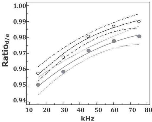
Figure 3 The branch of parabola concerning the  $\text{Ratio}_{d/a}$  versus the  $f_{step}$  relationship is shown as a black dashed line with the 95% confidence interval and the empty circles are the relationship's measured values. The branch of parabola concerning the  $\text{Ratio}_{d,le/a}$  versus the  $f_{step}$  relationship is shown as a grey continuous line with the 95% confidence interval and the full circles being the relationship's measured values.
