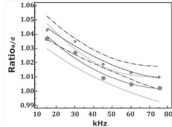
Figure 4. The branch of parabola concerning the  $\text{Ratio}_{a/d}$  versus the  $f_{step}$  relationship is shown as a black dashed line with the 95% confidence interval and empty circles are the relationship's measured values. The branch of parabola concerning the  $\text{Ratio}_{a,le/d}$  versus the  $f_{step}$  relationship is shown as a grey continuous line with the 95% confidence interval and full circles being the relationship's measured values.
