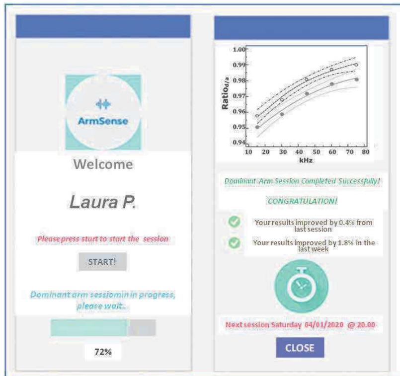
Figure 5 Representation, on an Android based smartphone, of two screens of the *ARMSense* application. On the left there is the main screen application and on the right is the screen with the Graphical User Interface (GUI) of the application.
