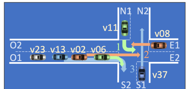
Figure 6: Example of three legal actions: action 1 allows the vehicle v11 from the southbound street and the vehicle v06 from the eastbound street to move simultaneously, followed by action 2 which dictates that v02 crosses, together with the westbound one v08; eventually, action 3 allows the northbound vehicle v37 to move together with v13 turning right.
