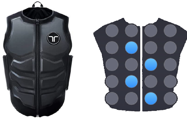
Fig. 4.26 Wearable and portable haptic suit with 40 vibration motors.
