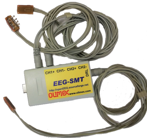
Fig. 2.1 The Olimex EEG-SMT acquisition board with two active dry electrodes connected to channel 1 for a single-channel differential acquisition and a passive dry electrode connected to “drive right leg” (DRL) reference terminal.
