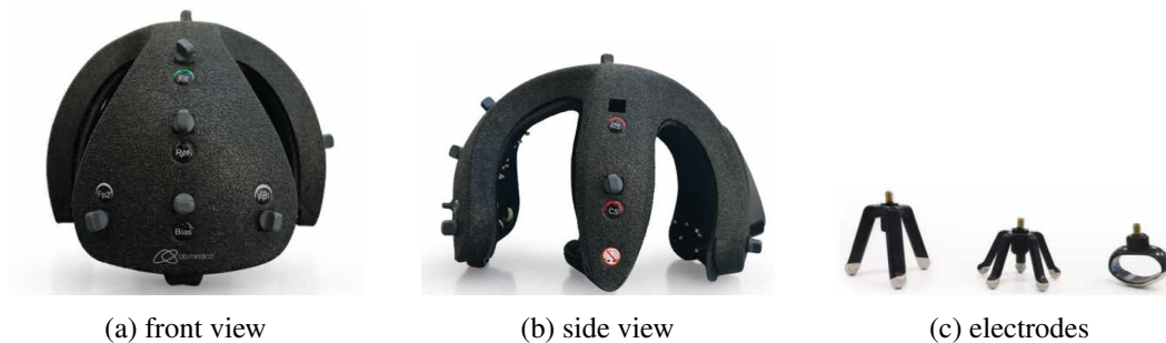
Fig. 2.2 The EEG cap Helm8 by ab-medica with ten dry electrodes in different shapes and bluetooth connection to ensure high wearability and portability.
