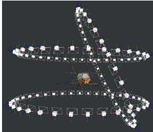
Fig. 5.1 Point cloud obtained after the Structure from Motion step with camera positions, represented in white.
