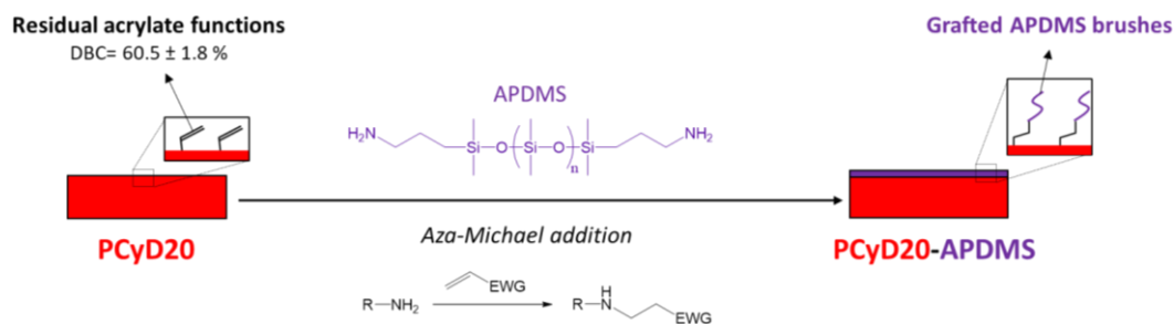
Figure 4.2. Schematic representation of the surface-grafting of A-PDMS brushes onto PCyD20 following the path of an aza-Michael reaction.
