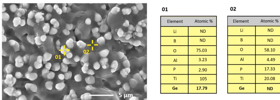
**Fig. 5.** EDS analysis performed on powder sintered LAGTPB (LAGTPB-s) to evaluate the composition of the bright areas observed on its non-polished surface. The analysis was carried out in high vacuum and at a voltage of 15 kV.
