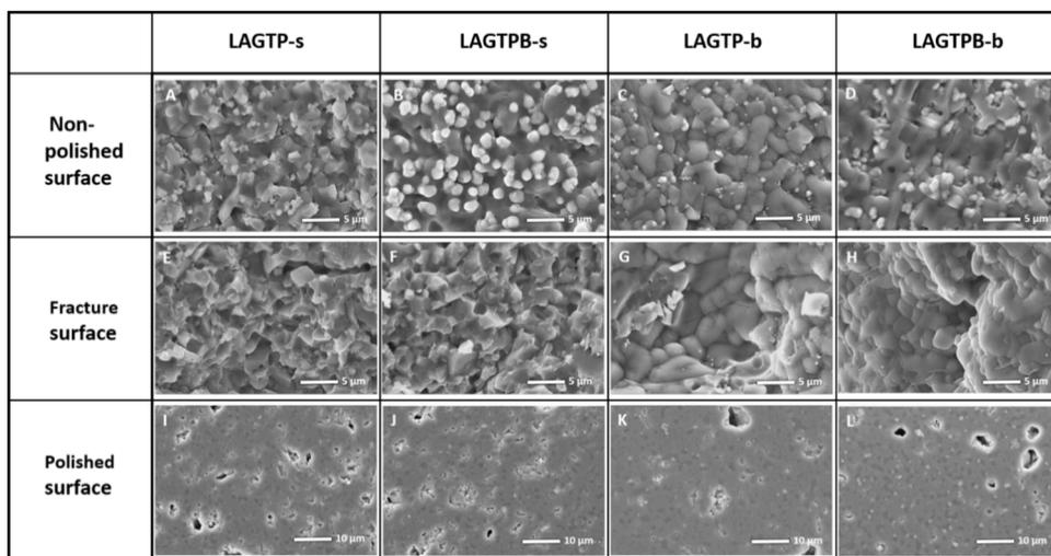
**Fig. 4.** SEM micrographs of non-polished, fracture and polished surfaces of sintered and bulk heat-treated LAGTP and LAGTPB. From above: sintered LAGTP-s (A,E,I) and LAGTPB-s (B,F,J), bulk heat treated LAGTP-b (C,G,K) and LAGTPB-b (D,H,L). From the left: non-polished (A,B,C,D), fracture (E,F,G,H) and polished (I,J,K, L) surfaces.
