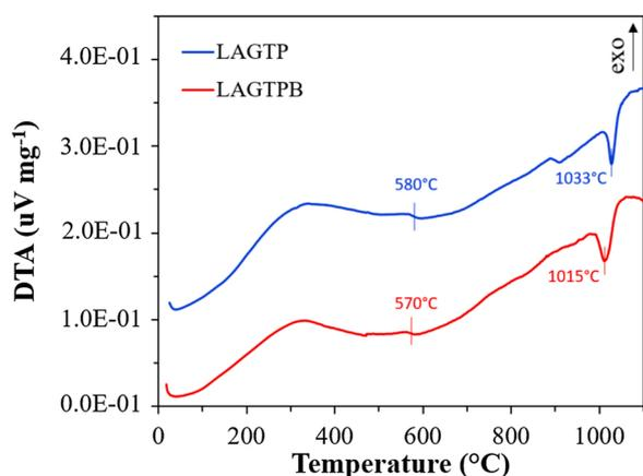
Fig. 1. DTA curves of as-casted LAGTP and LAGTPB.
