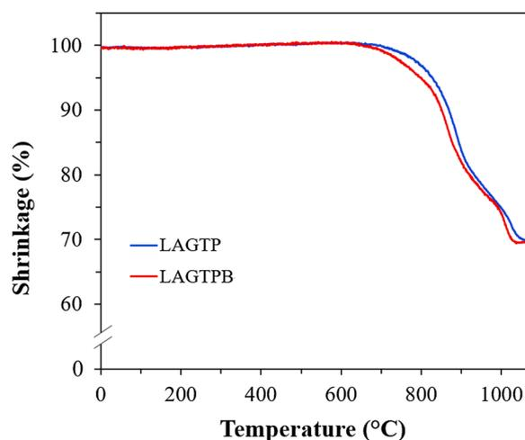
Fig. 2. HSM curves of as-casted LAGTP and LAGTPB upon a scanning rate of 10 °C min<sup>-1</sup>.
