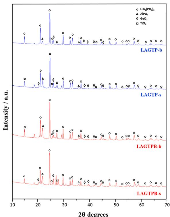
Fig. 3. XRD spectra of LAGTP and LAGTPB after powder sintering (-s) or bulk heat treatment (-b). The XRD patterns were recorded in the  $2\theta$  range of  $10\text{--}70^\circ$  at a voltage of 40 kV and a current of 40 mA.
