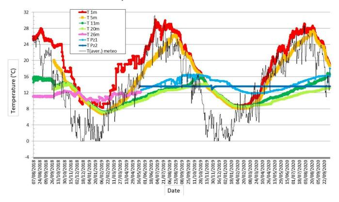
Figure 7. Water temperatures (T;  $^{\circ}$ C) from over more than 2 years of monitoring at different depths inside the "Provana" quarry lake (red, yellow, light green, dark green, and pink lines), groundwater temperatures measured at Pz1 (light blue) and Pz2 (dark blue); the average daily atmospheric temperature (black line).
