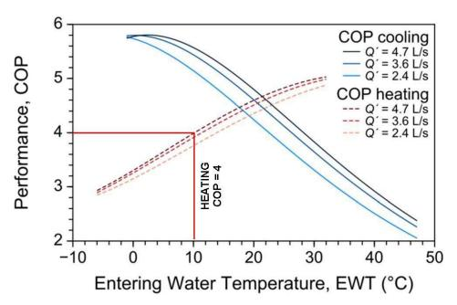
**Figure 6.** Coefficient of performance (COP) of a water-to-air heat pump system in heating and cooling mode according to the temperature and flow rate of the water entering the system [26].
