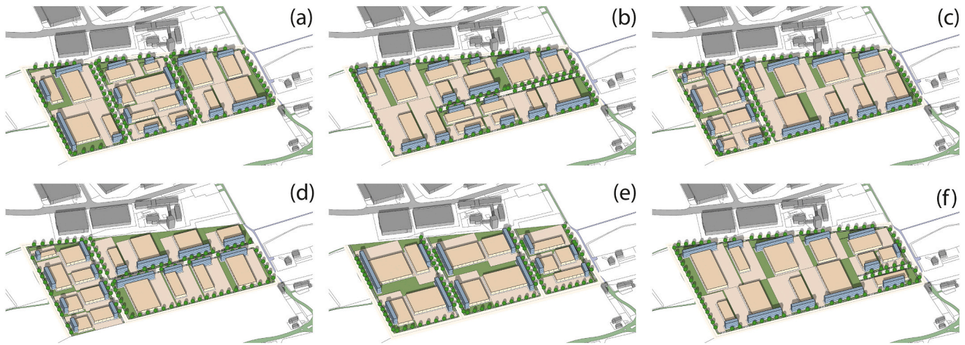
Fig. 5. The system rapidly generates and visualises the compliant layouts. Six Pareto-optimal choices of production out of the Pareto front, providing an outlook on DMs' set of criteria. In (a) and (b) every single land plot retains the same surface, dimensions and position, but the road pattern varies, and consequently the building orientation. In (c) and (d) the plots retain the same surface of (a) and (b), but their dimensions and position vary; new road patterns and EIP layouts are generated. (e) and (f) differ in plots' number, area, dimensions and position; the road pattern and EIP layout change accordingly.
