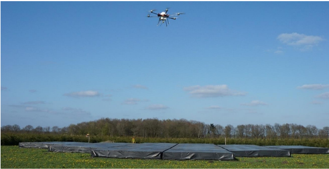
Fig. 1. The UAV after take-off is reaching the first waypoint to perform the required scan path over a LOFAR HBA array of the CS302 station. The array size is about 30 m.
