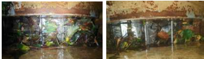
Figure 2. Visual inspections and accumulation of organic vegetal bodies: immediately after operation (left) and after few minutes of inactivity (right).
