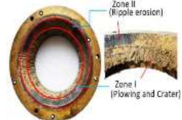
Figure 6. Wear on nozzle ring (Din and Harmain 2020)
