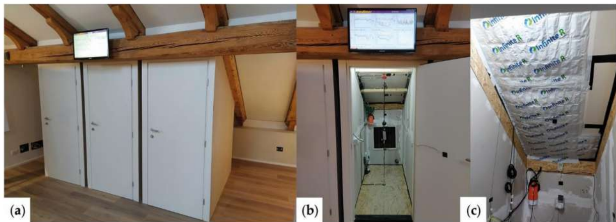
Figure 2. (a) The TRIS apparatus; (b) View of the internal space of a cell; (c) Installation of the Infinite R™ panels.
