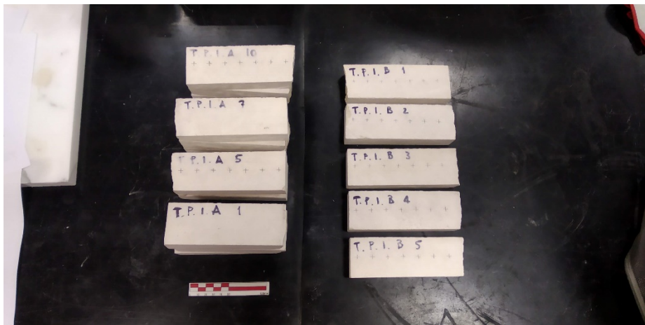
Figure 8: The specimens cut from the chiancarella gathered from Trullo Palmullo (Martina Franca). They are divided into group TPI A and TPI B: TPI A specimens come from the unaltered part of the chiancarella, while TPI B come from the superficially weathered half.
