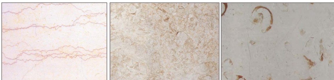
Figure 5: From left to right Filetto Rosso Jonico; Perlato Svevo; Cocciolato ornamental stones. Fossil dimensions can range between 5 and 20 mm. (Cotecchia et al., 1982).
