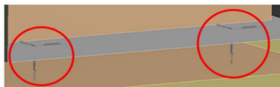
Figure 5. Anti-vibrating supports FEM modelling.
