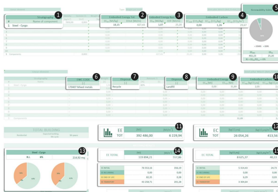
Figure 3. The figure shows the EURECA main results: numbers 1 to 5 refer to EE, EC, and RI of the material, or the building system; numbers 6 to 10 refer to EE and EC of the materials matched to the EU waste code; numbers 11 to 15 refer to EE, EC calculated for the building as a whole.
