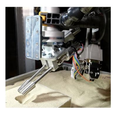
**Figure 3.20** The Dual-Rasp sampling system combines the capability to sample a wide range of surface material strengths with the advantage to require low average preload.
