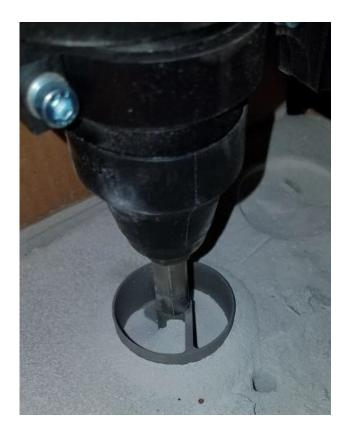
Figure 3.6 Test of the full-face drill bit with linear teeth arrays.
