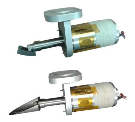
**Figure 3.17** Prototype of the ultrasonic sampling system provided with two different types of scoop. Curved (Top) and straight (Bottom). The curved scoop helped the mitigation of some drawbacks of the straight version, namely the higher reactive loads and the higher difficulty to handle the sample during sample chain steps.
