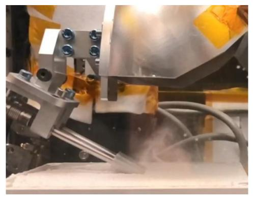
**Figure 4.61** Sample transport of approximately 10  $\mu$ m particles in 1 atm conditions.
