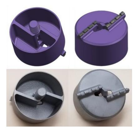
Figure 3.5 Front face drill bit with linear teeth array design (Top) and 3D printed metal test bits (Bottom).
