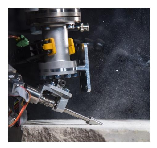
Figure 3.21 The Dual-Rasp involved in sampling operations.
