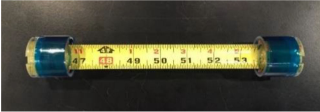
Figure 13. A 170 mm sample of commercial tape-spring. Figure elaborated from Ref. [39].
