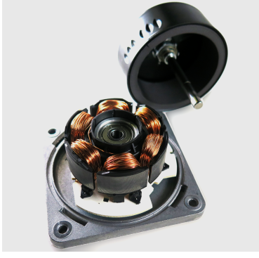
Fig. 1: Motor under test with disassembled outer rotor.
