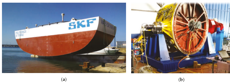
Figure 1. ISWEC device installed in Pantelleria island (Sicily, Italy): (a) ISWEC Pantelleria hull; (b) ISWEC Pantelleria gyroscope.
