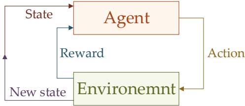
Figure 2. Block diagram of reinforcement learning (RL) control.
