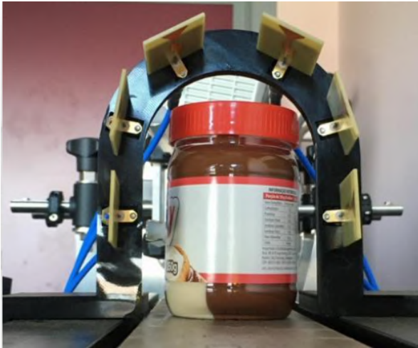
Fig. 1. Antennas array surrounding the item to inspect
