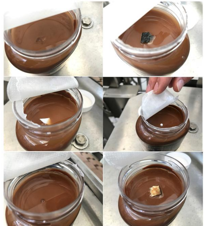
Fig. 4. Initial placement of different types of intrusions inside the tested products
