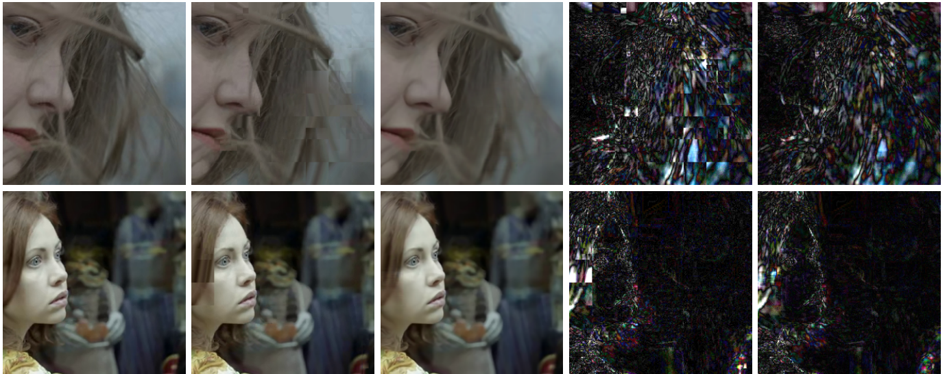
Fig. 4. Frame comparison, from left to right: original frame, HEVC MC frame, enhanced MC frame, residual using HEVC MC frame, residual using enhanced frame. The enhancement scheme manages to remove most of the block-shaped artifacts present in the HEVC MC frames.
