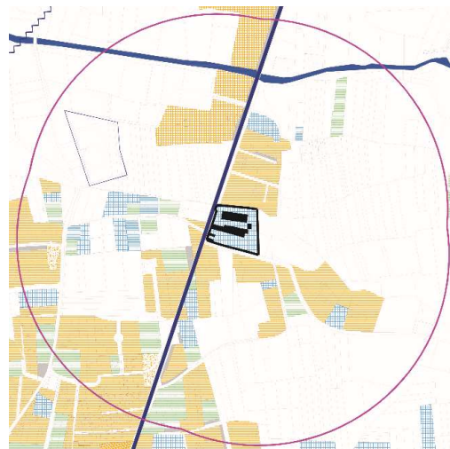
Figure 4: Example of buffer zone for a Seveso plant
