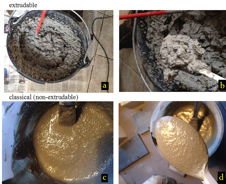
Fig. 1. Qualitative comparison of cohesion and viscosity of extrudable (a, b) and classical (c, d) foamed concrete at the fresh state (specimen preparation with equal target dry density of 600 \text{ kg/m}^3 ).
