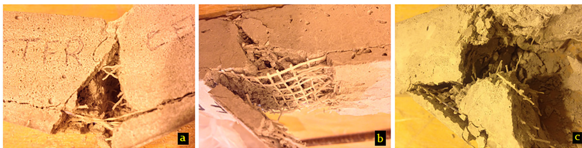
Fig. 21. Photographs at failure of foamed concrete beams cured in cellophane: a) close-up detail at the mid-span beam soffit; b) interaction between short polymer fibers and glass-fiber bi-directional grid reinforcement; c) detail of the rupture zone with concrete detachment.
