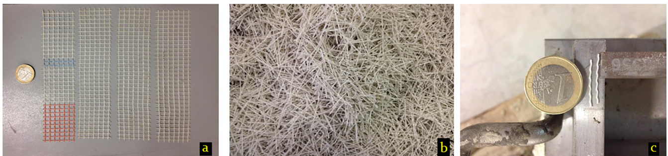
Fig. 3. Glass fiber reinforcement bi-directional grid (a) and short polymer fibers (b, c).
