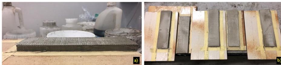
**Figure 2.** Final samples of FRIL-panels: a) removal of lateral guides and assessment of the self-supporting capacity immediately after the pouring phase; b) series of 5 FRIL-panels left at environmental conditions (pre-curing phase) for 12 hours.
