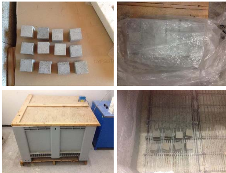
Figure 1 Curing conditions of the tested specimens in air at environmental temperature (top left), wrapped in a cellophane sheet at environmental temperature (top right), and in water at controlled temperature (bottom left and right)
