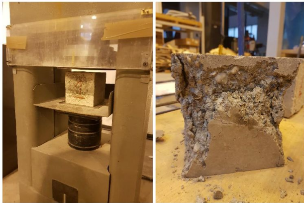
Figure 6: Compression test in accordance with UNI EN 12390-4 on concrete cube sample
