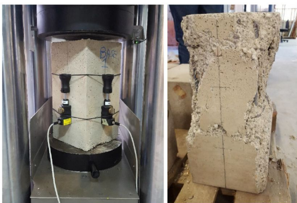
Figure 8: Compression test on sample of reinforced concrete column: placement of strain gauges (left) and typical failure mode (right)
