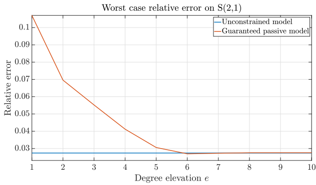
FIGURE 13. Coupled transmission line. Relative error \epsilon_{2,1} for the passive models based on different degree elevations, compared to the error of the model obtained without enforcing any passivity constraint.
