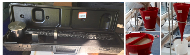
Fig. 3. Mud balance (on the left) and the Marsh cone (on the right). Pictures modified from [30].
