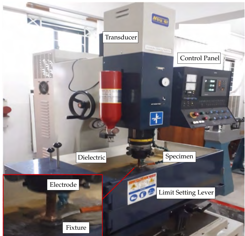
Figure 2. Experimental setup for EDM.
